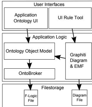
**Fig. 1.** Overview of the architecture of the UI Integration Tool.
