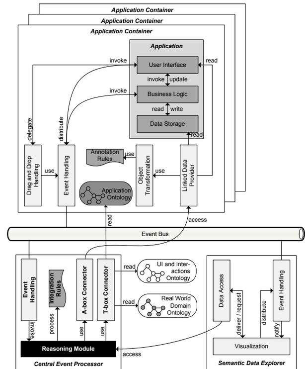
**Figure 1. Overview on the architecture of our framework. Each integrated application runs in a container, which provides information as linked data and is connected to a message exchange bus. The Semantic Data Explorer visualizes that data by directly interfacing a reasoner.**
