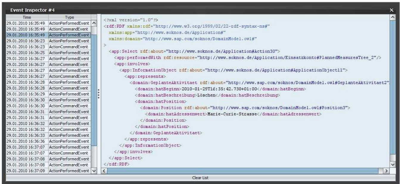
Figure 3. Events are exchanged in a common RDF-XML representation. Developers may use the event inspector to analyze the event exchange in detail.
